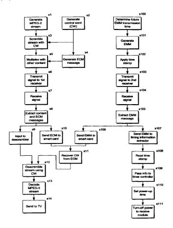
(57) Abstract: A conditional access system in which entilement management messages (EMMs) sent to a receiver include transmission time information for future EMMs. The transmission time information is used at the receiver to control the receiver so that it is powered on only when required to receive the future EMMs.
